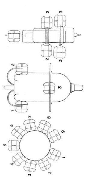
DIAGRAM OF SPECIAL VALVE HOLDERS (showing pin connections viewed from above). What follows in the manual is 106 pages of valve set up data for the CT160 which I have not scanned!
